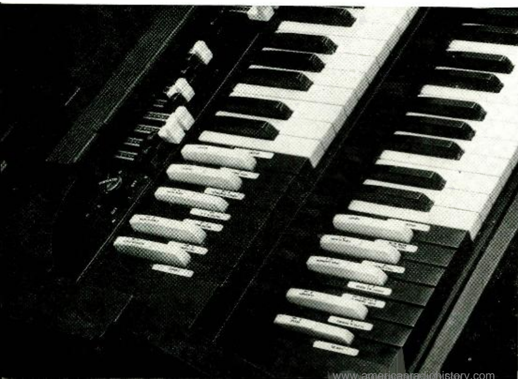
Fig. 1. Detailed view showing principal controls. Precept keys are reversed in color to avoid confusion with playing keys.
