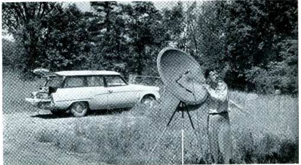
Dr. William Gunn, field secretary of the Federation of Ontario Naturalists, adjusts the parabolic microphone reflector to "focus" on a feathered songster. The reflector strengthens the primary signal, permitting reduced recording level and lower background noise.
