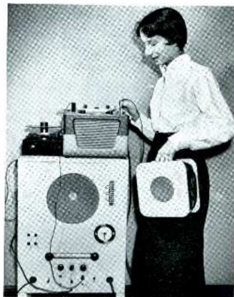
Lois Luebke (my oldest daughter) demonstrates our prize gadget, the "rambling speaker." The speaker itself forms the reel for the long wire that enables us to listen to a tape in almost any room of the house. There is never any messy left-over wire because only as much as is needed is taken off the reel. The speaker is equipped with a "closed circuit" jack that permits the use of earphones.
