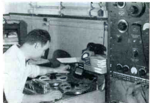
Precision test equipment measures the frequency response of Audiotape production samples.
