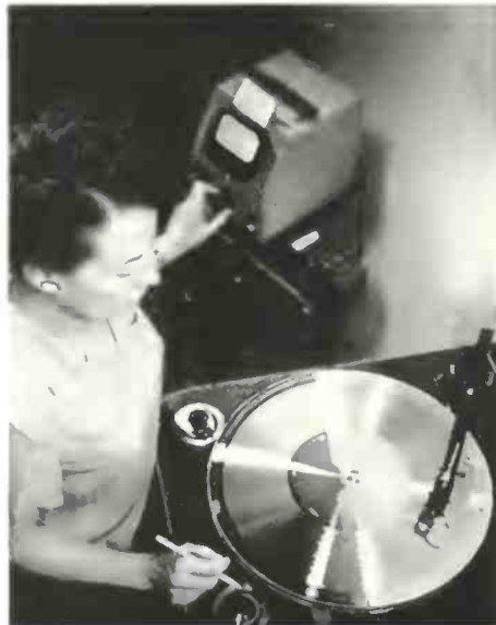
Complete audio testing of all metal "mothers" is just one of Allied's many exacting quality-control measures. In addition, every tenth pressing is played all the way through, to catch any imperfections which might possibly develop in the matrix or stamper.
