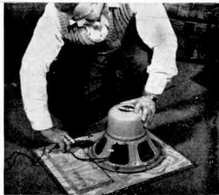
Above: Mounting a speaker on a baffle board. Screws should be tightened uniformly to avoid warping speaker frame. Left: Technicians Richard Hilton and Theodore Osborne reassemble an enclosure after testing it
