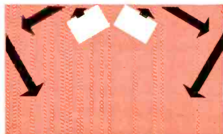
An unusual arrangement. Sound is reflected from the back wall to the two adjacent walls, then finally to the listener
