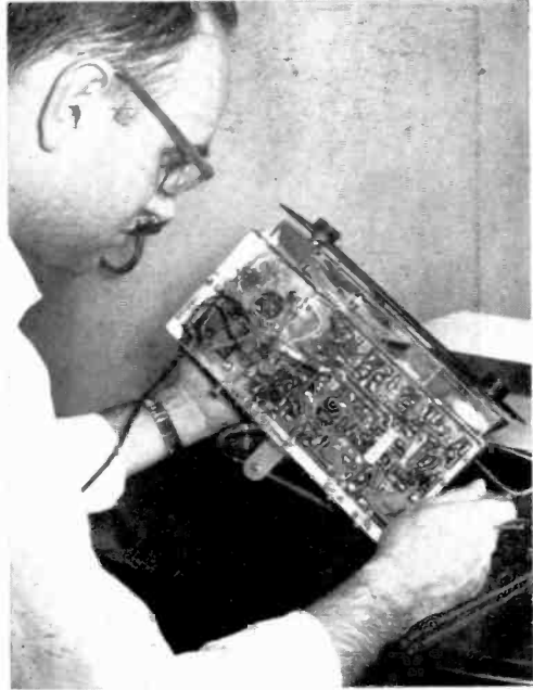
Above: Parts mounted on printed-circuit board should be checked before connections are made. Right: Underside of printed circuit board used in Allied tuner kit
