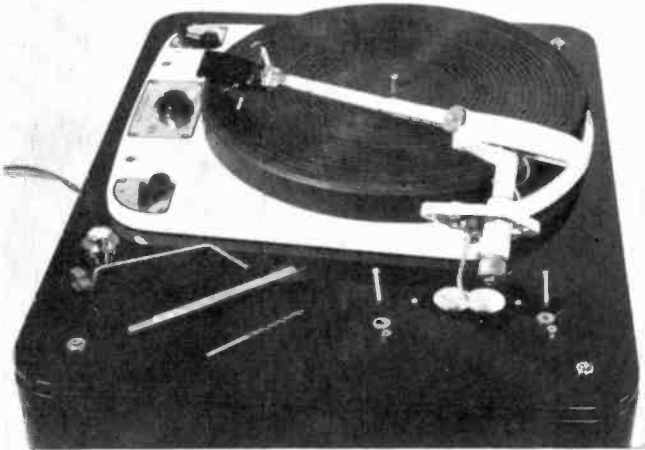
Correctly positioned holes have been drilled in the turntable base to accept the tone arm and mounting hardware
