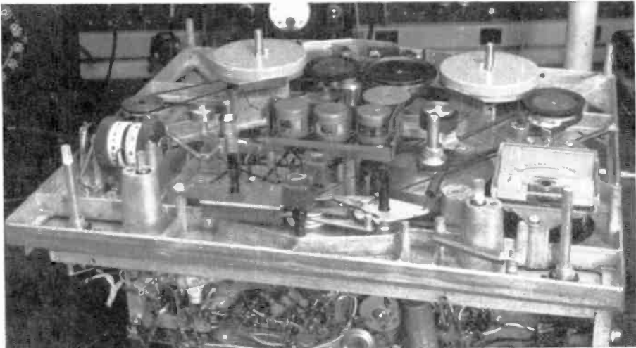
Above: Ampex 601 monaural tape recorder. Below: Ampex "A" series tape deck with cover removed. Note erase, record, and in-line stereophonic playback heads
