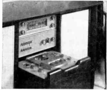
Opposite page: Different types of tape-recorder heads. Right: Experimental tape magazine unit incorporated into a stereophonic radio-phonotape console by Ampex Audio
