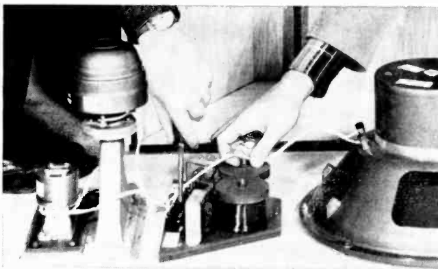
The crossover network employed in the Klipschorn loudspeaker system uses inductances and capacitors to divide the different frequency ranges
