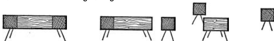
Moving away from the stereogram. Separating one speaker would aid stereo accuracy but have little further effect. Separating both speakers is fundamental in hi-fi.
