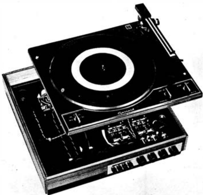
Fig 39. An amplifier and turntable plinth assembly using the high-quality Garrard AP 75 automatic single-record-playing turntable and arm assembly on a plinth into which Sinclair stereo pre-amplifier and power-amplifier modules have been assembled. The modules of Figs 24-9 may be used or alternative power units may be fitted to give power output ratings of over 40 watts per channel. The AP 75 arm gives a micro-adjustment of tracking weight down to below 2 g with side thrust compensation. Automatic record-starting, groove-positioning and automatic lowering, raising and stop are provided as well as a pause-control.
