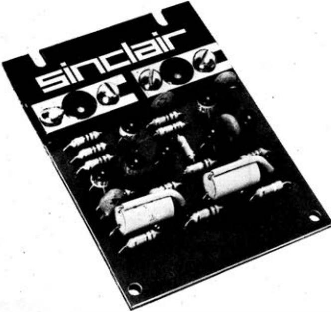
Fig 25. A picture of the power-amplifier module of Fig 24. The printed circuit board is 2\frac{3}{8} by 2\frac{1}{2} in. The power output transistors at the top of the picture are mounted on a matt black heat sink large enough to dissipate the heat generated by moderate music powers. Larger powers may be dissipated if the heat sink is mounted intimately in contact with a larger metal chassis etc.
