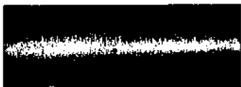
FIG. 11/2.—Oscillogram of needle scratch produced in wide range two-speaker system. Shellac record, groove diameter 10 ins. 78 rpm, 400 ohms magnetic pick-up, without transformer.
