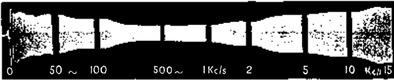
FIG. 17/6.—Response of original version of Garner Amplifier with pre-amp. Controls set for maximum bass and full top lift. There are indications of phase shift usually associated with tone control circuits.
