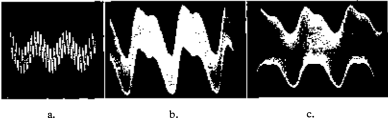
FIG. 1/7A.—Oscillograms to illustrate intermodulation effects produced in loudspeakers.
