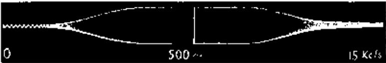
FIG. 17/7.—Controls set for minimum bass and minimum top. Otherwise same as Fig. 17/6.
