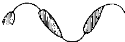
FIG. 5/2.—Oscillogram of shock-excited parasitic oscillation of extremely high frequency, carried on 50 cycle mains hum.
