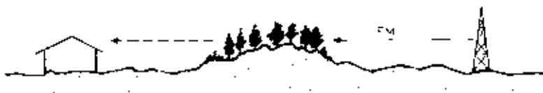
Fig. 5.16 Even in the service area the f.m. signal can be attenuated by having to pass through a wooded area as this diagram shows.
