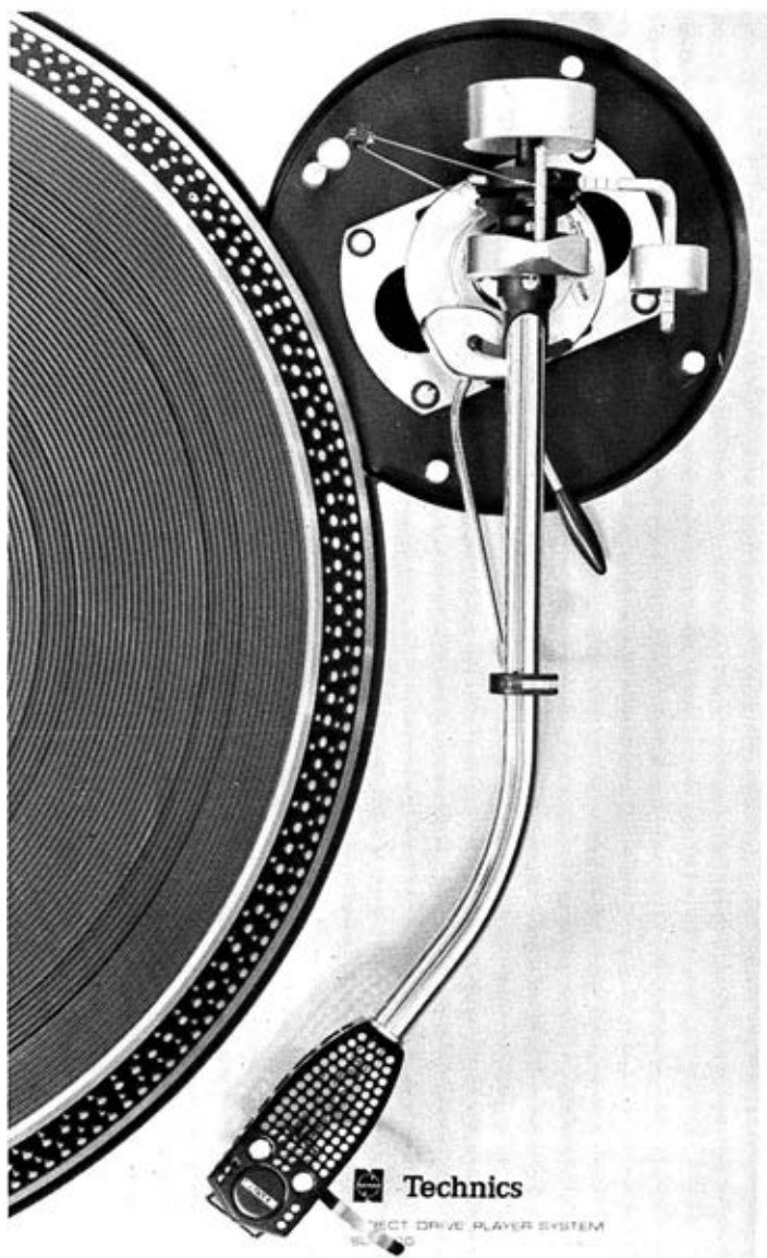
The SME pickup arm seen from above. Note stroboscopic markings on periphery of turntable ( Photograph courtesy of SME Ltd, Steyning, Sussex )
