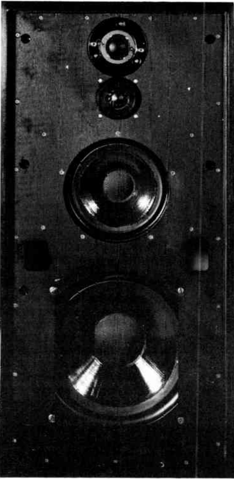
Figure 6.3 A four-way vertical-in-line system (18 dB/octave electrical crossover with controlled listening axis) (BC3, Courtesy of Spendor Ltd.)
