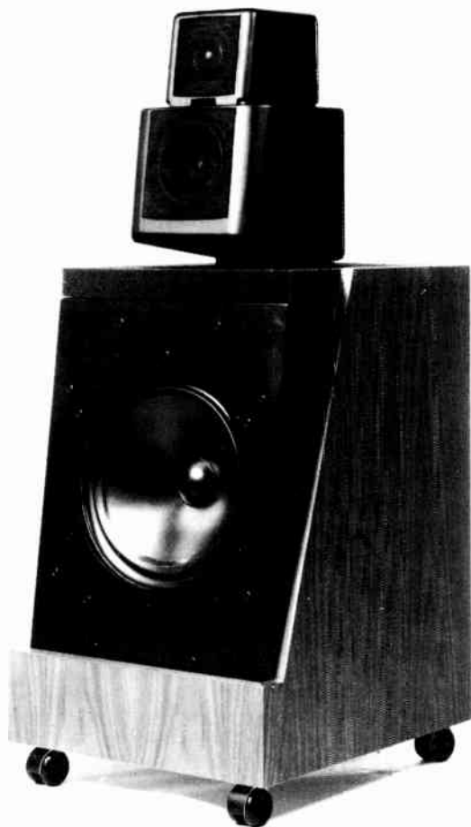
Figure 6.2 (c) A three-way system with time aligned drivers, 24 dB/octave, crossover (acoustic) and low diffraction enclosure forms (Courtesy KEF Electronics)
