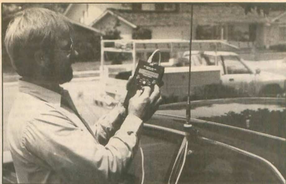
The MFJ SWR analyzer is easy to use to tune your HF whip.
