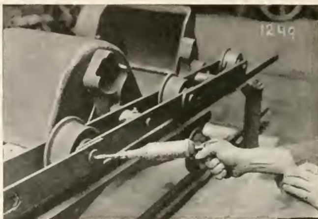
A posed picture showing method of lubricating a conveyor chain. The hand, oil gun and chain pin have been spotlighted to make them stand out. A short exposure with a fairly large lens opening
