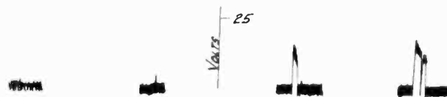
FIG. 6—CONTACT DROP OBTAINED WITH FOUR DIFFERENT BRUSH AND BRUSH HOLDER ARRANGEMENTS
