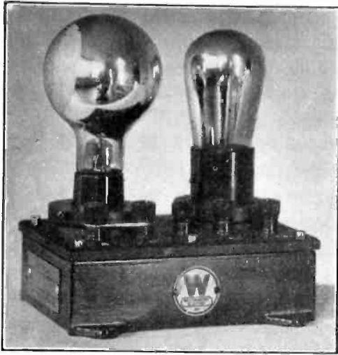
FIG. 4—ILLUSTRATION PHOTO-CELL AMPLIFIER UNIT SHOWING A 2½-IN. DIAMETER PHOTO CELL AND A STANDARD 201-A RADIO TUBE IN POSITION ON THE PANEL
