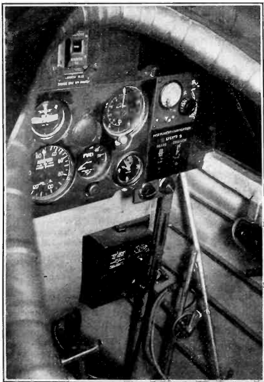
FIG. 4—INSTRUMENT BOARD WITH BEACON INDICATOR MOUNTED ABOVE THE OTHER INSTRUMENTS
