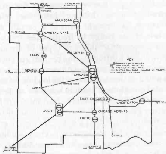
FIG. 7—LOCATION OF TELEPHONE REPEATER STATIONS AND THEIR RELATION TO THE TOLL CABLE NETWORK IN THE CHICAGO SUBURBAN AREA
