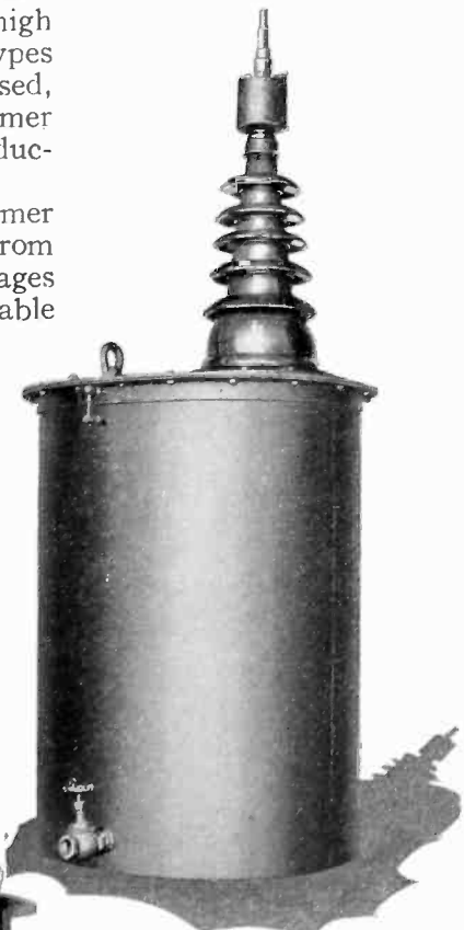
150,000 volt testing transformer with one end grounded
