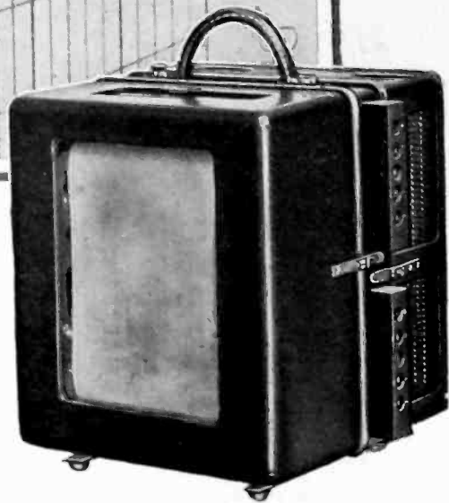
Type CP-4 5-amp. 110/220/550 self-contained Polyphase Wattmeter.
