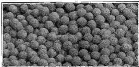
FIG. 1—LEAD PEROXIDE PELLETS BEFORE BEING COATED WITH AN INSULATING POWDER
