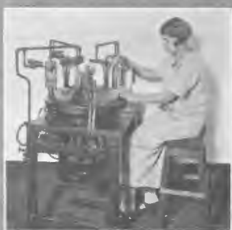
Valves in Course of Manufacture at the A.W.A. Valve Works, Sydney
