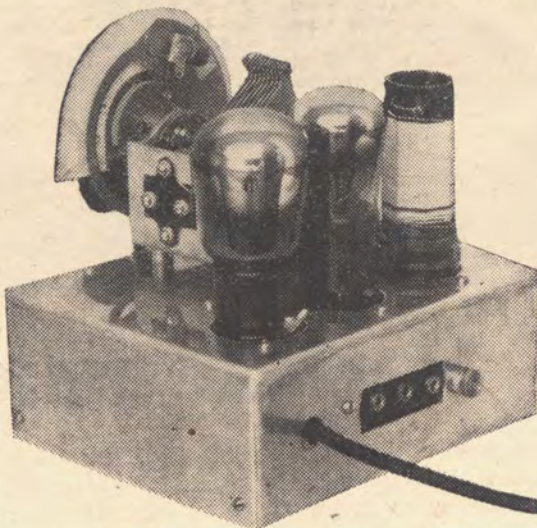
A rear view of the receiver showing the aerial-earth and output terminals mounted on the side of the chassis.
