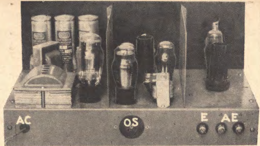
A rear view of the chassis which shows clearly the division of the three main sections of the receiver.
