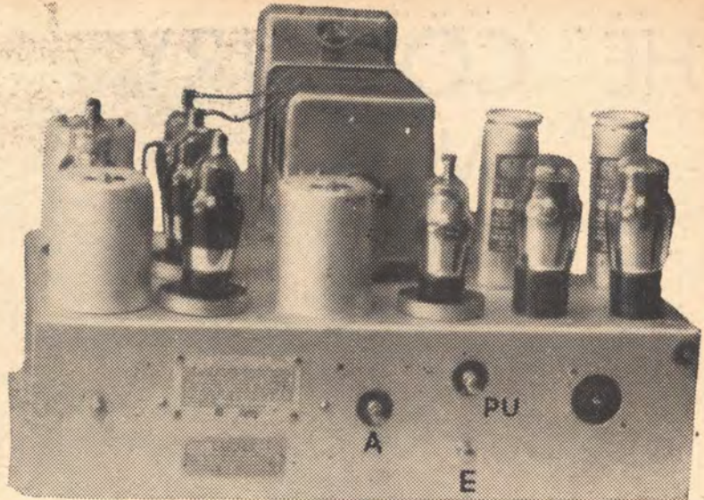
A rear view of the receiver showing the disposition of the pick-up, aerial, and earth terminals.
