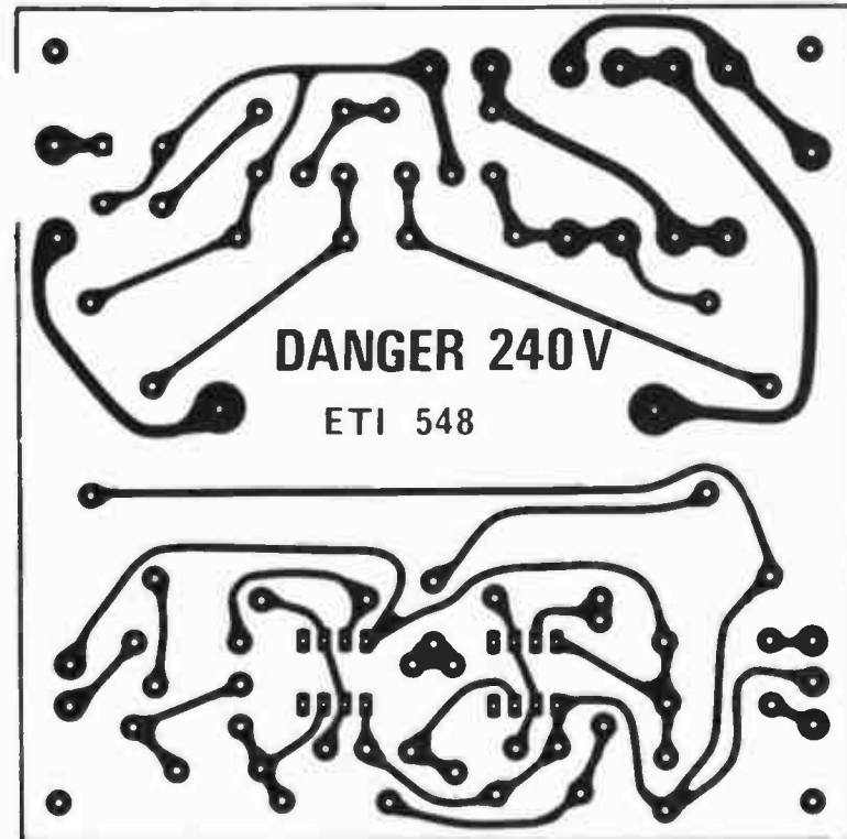
Fig. 4. Printed circuit layout. Full size 100 x 100 mm. Material used MUST be fibre glass due to the heat generated by R1.
