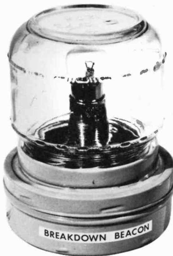
Inside view of the completed unit. Note the plastic disc used to replace the normal airtight seal of the jar.
