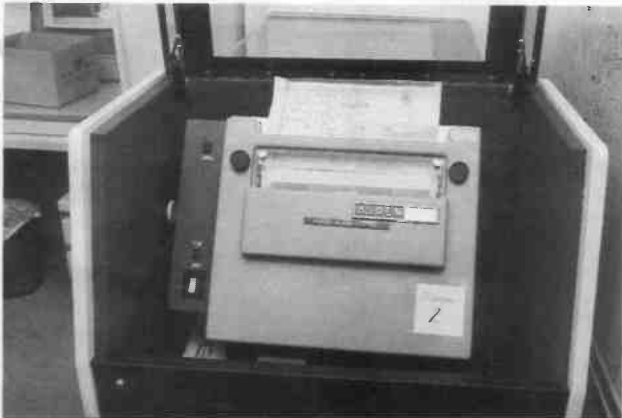
A mechanical weather-fax machine at the Hobart Weather Bureau.
