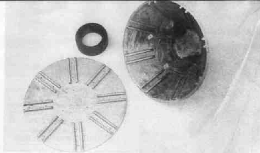
These are the pieces that make up the disccone hub supplied by Ashpoint Industries. At front left is the disc piece and at top right, the cone piece; both are sturdy aluminium castings. The ring at the rear is the acetal plastic insulator. Note the fillets in both castings, used to locate the 9.5mm diameter aluminium tubing elements. Note, also, the 'dimples' in the disc piece casting which are used to locate the various holes to be drilled, thus making your job easier. There are also dimples in the flat section on the top of the cone piece casting.
