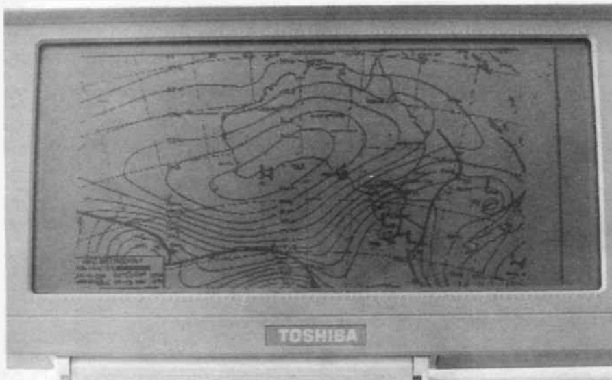
A sample fax picture of the kind produced by the author's Listening Post II software, on a laptop's LCD screen...
