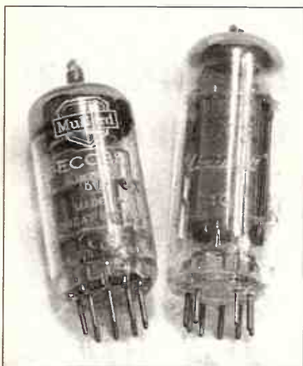
Younger triodes you will encounter: two 9-pin miniature all-glass valves; an ECC88 (encountered in audio and RF circuits) is at left and a 6CG7 (encountered in audio and TV circuitry) is at right.
