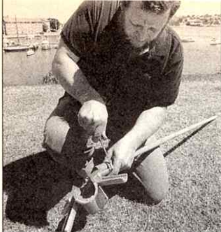
The sealed spreaders are secured in the hub piece arms using hose clamps.
