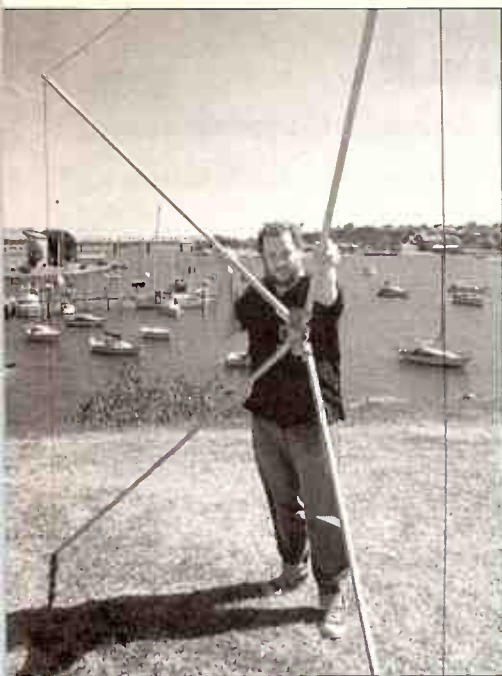
One completed quad element. Now for the next one, to complete the cubical quad.
