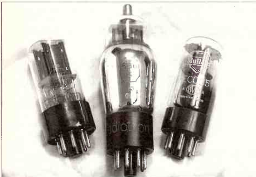
Older triodes you will encounter: in the centre is a widely-used old triode, the 6B6. At left is a somewhat younger twin-triode, the ECC35.
