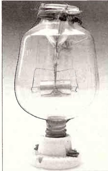
A glorious old triode! Such are rarities, but triode circuit building blocks were developed using devices such as this. The filament connections run down the bulb to the Edison screw base; the grid and anode (plate) connections are made to wire brought out at the top.
