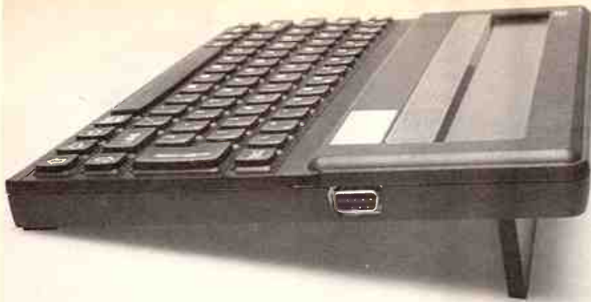
Side-on view, showing the foot which folds down from the rear of the case. The connector you can see there is the DB9 RS232 serial interface.
