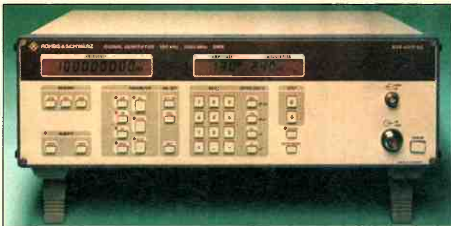
This Rohde & Schwarz RF signal generator, model SMX, is one of their economy instruments. It covers 100 kHz to 1000 MHz in frequency and -137 to +13 dBm output level. AM, FM, pulse and two-tone modulation is included.
