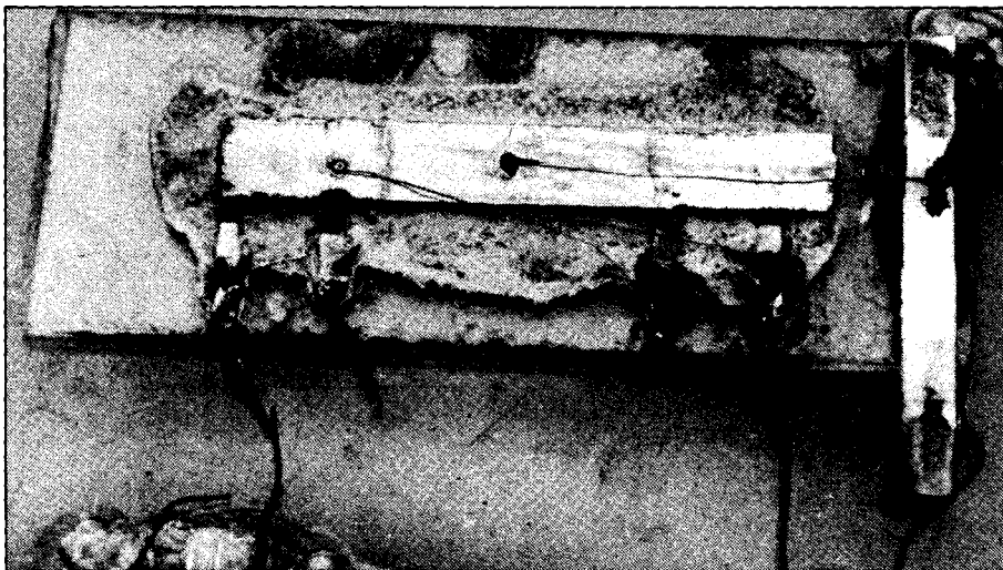
A 1958 photo of Jack Kilby's original device. This primitive working model validated Kilby's premise that both active and passive components could be composed of the same semiconducting material.
