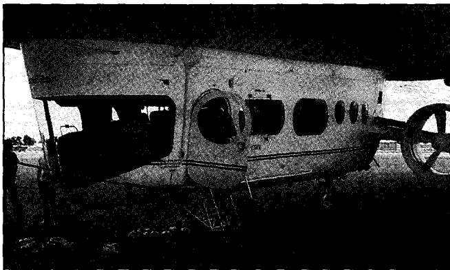
Gondola showing entry door, cockpit, engine nacelle and castoring undercarriage wheel.
