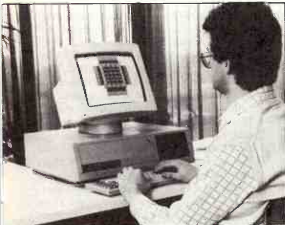
The LASARRAY Design System allows the easy development of customized chips. The design data are directly used as input for the Direct-Write Laser in the LASARRAY Processing System. Photo: LASARRAY
