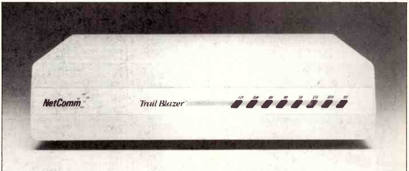
Netcomm's Trailblazer is one of the fastest locally produced modems, running at up to 18 000 bits per second. It uses a multi-carrier modulation scheme, advanced digital signal processing and packet technologies to dramatically increase the throughput using ordinary Telecom lines. A unique feature is real time analysis of the bandwidth of the line, which determines the usable carriers, how many bits per second given the line conditions and what data flows exist. In fact, it can send data only in the good parts of the line and completely ignore impaired frequencies.
