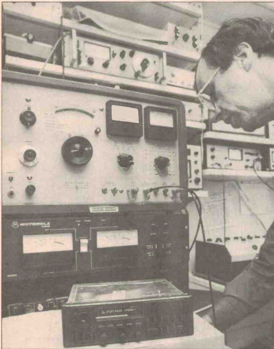
Testing at the House of Challs. The Eurovox MC2360E is connected to an HP AM signal generator (the big gadget on top). This device has an AM stereo modulator, transmitter exciter and low powered transmitter output. It enables measurements of AM stereo frequency response and channel separation to be taken.
