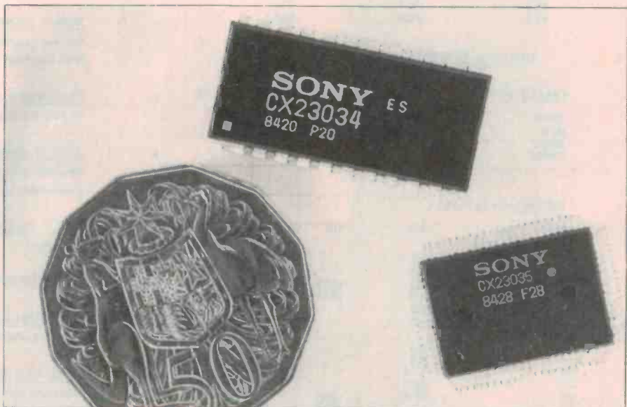
Sony has reduced most of the electronics in the D50 CD player to just these two ICs.
