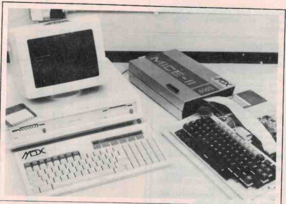
Figure 6. MICE can be operated from a VDU, or, as shown, from a computer system running a driver routine.
