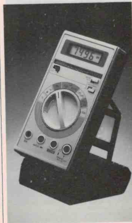
Aaron MM210. The colour coordination in this little meter is terrific, but the case feels very flimsy. It's main advantage is 1G input resistance, which, for the price, is unbeatable. The distributor is Neotronics.
