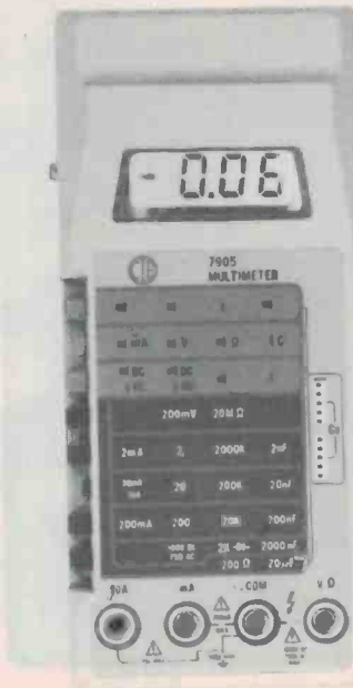
CIE 7905. One of the better Taiwanese-made meters. It has a stylish case and sits in the middle of the model range, both in terms of price and electrical performance. Note the capacitance tester on the right hand side. Distributed by Lamron.
