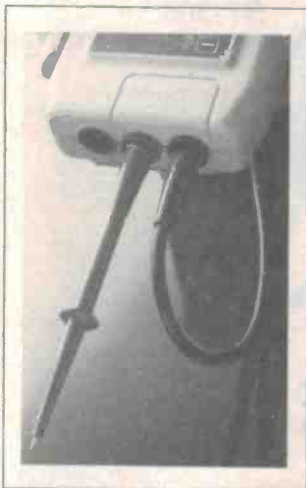
Avo 2001. One of the three DMMs available from Avo in this country courtesy of Electrical Equipment P/L of Sydney. It features very fast response time, in line sockets with a custom-built probe for single handed operation, and an audio warning of incorrect operation on the 10 A range. Although new and relatively unknown its name will probably excite interest even at $184.
