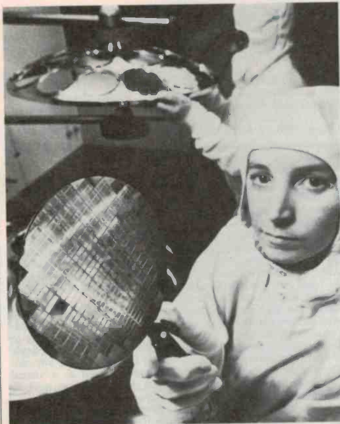
Karen Kaigle holds a silicon wafer. The wafer contains memory chips that can store more than one million bits of data. The wafer will eventually be diced into almost 100 individual chips.
