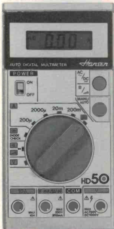
Hansen HD 50. A rather pricey meter from Japan, distributed by University Graham. It combines auto-ranging on volts and resistance with a comprehensive manual range function on current. The distributors should undoubtedly rewrite the manual.
