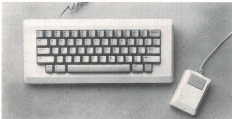
Drivers' position. The keyboard and the mouse — for driving Mac. The mouse's functions are not emulated on the keyboard. ▼
