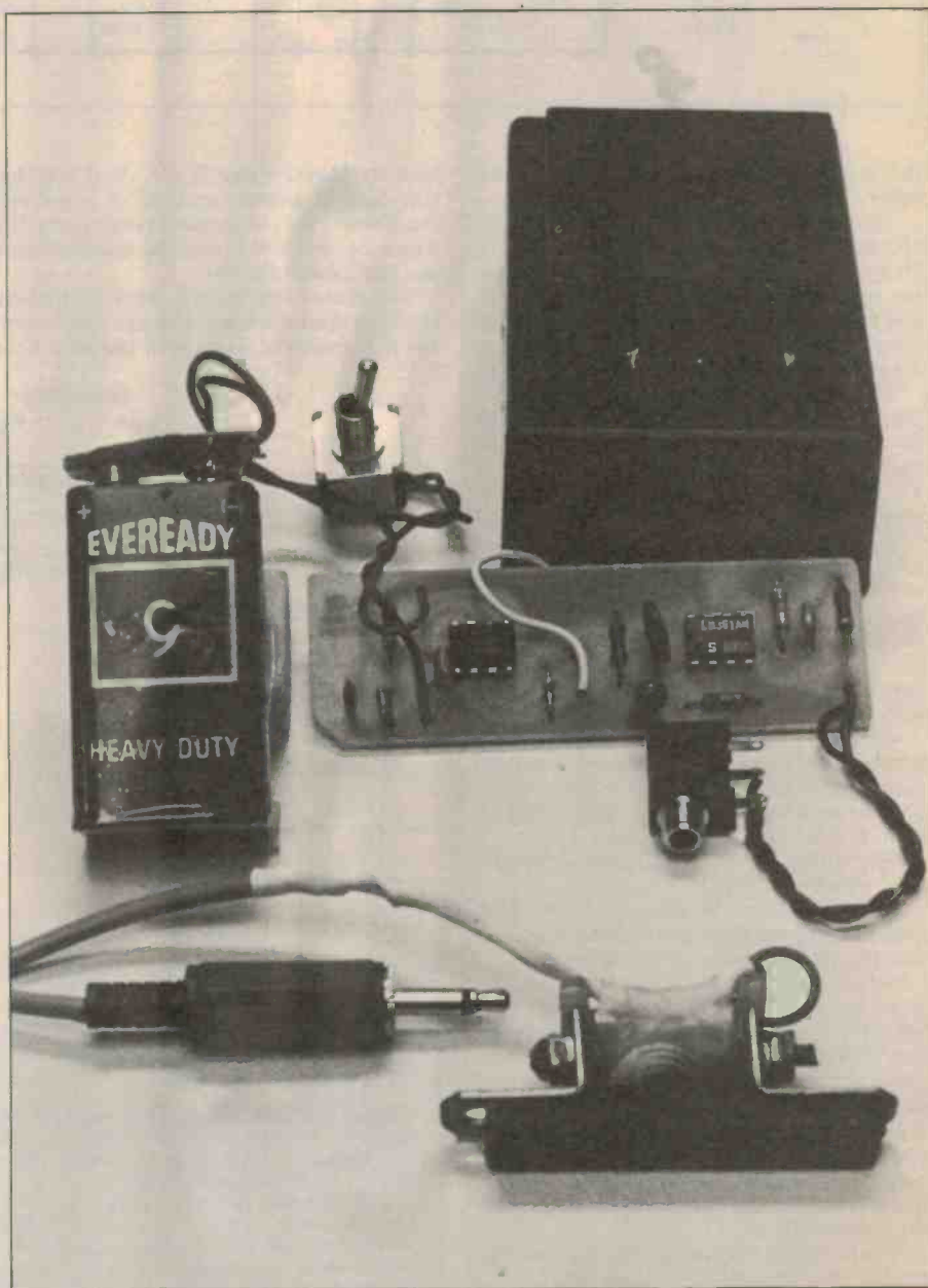
Neat and simple. All the bits for the Let Caller. There's not much to it, but it's certainly effective. The sensor coil is shown in the foreground. It mounts on the net cord (see diagram next page).
