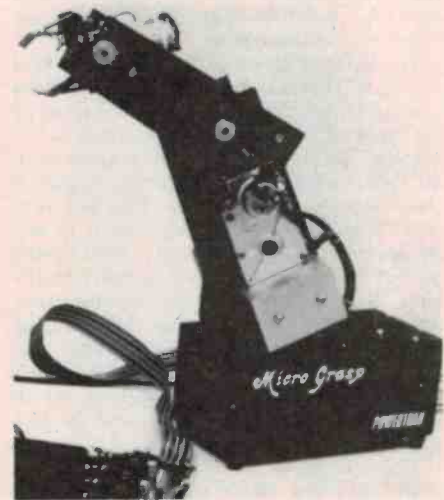
This'll grab you! The Micro-Grasp, a computer controlled robot arm project, scheduled to be described in April ETI, features four degrees of freedom, a motorised gripper and simple interfacing.
