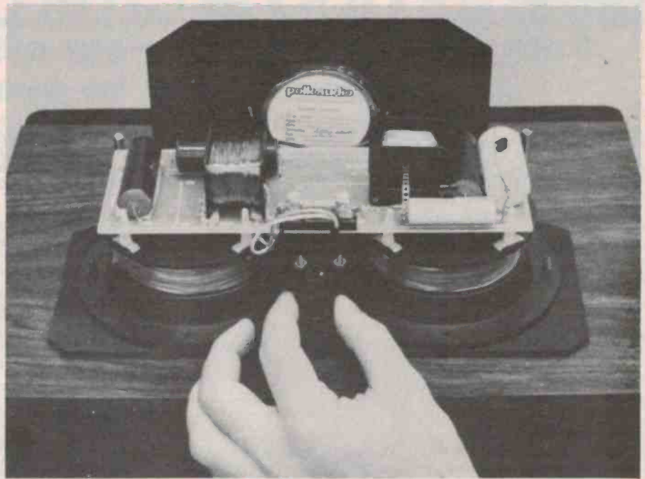
The crossover network and tweeter come as a single unit which mounts to the top of the bass enclosure and connects via a plug.
