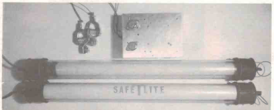
Our final prototype. We used two 20 W tubes housed in 'Safe-T-Lite' enclosures. Put protective plastic caps over the transistors to prevent shorts. One 'starter' wire (see circuit) can be seen wound around the top tube.
