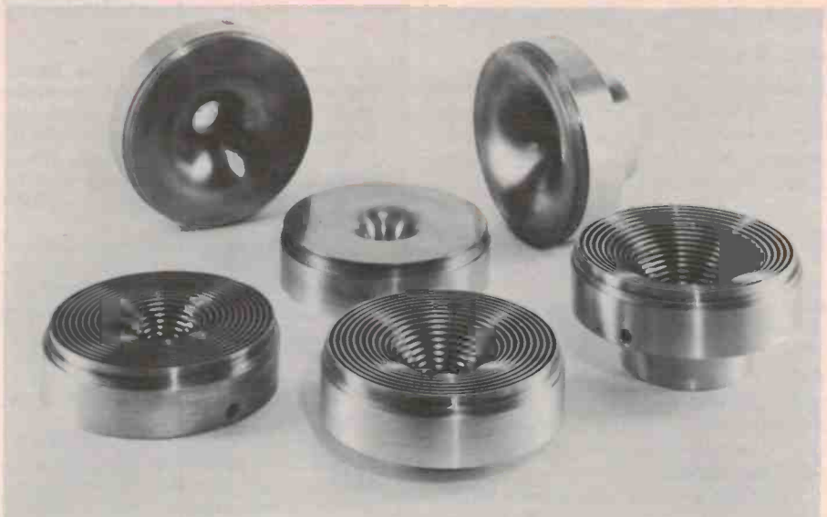
Flared corrugated horns, developed by the CSIRO Radiophysics Division, improve radiation pattern symmetry and provide low cross-polarisation with dish antennas — an important requirement in making accurate observations.
