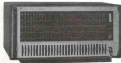
The first equaliser I ever saw was this 1/3-octave band spectrum shaper made by General Radio. It featured key-locked controls.
