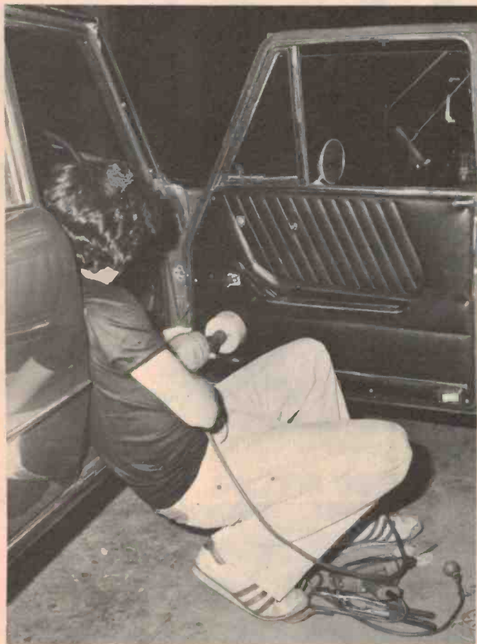
Speakers are best positioned so that sound output is not obscured to any great extent by seats or passenger's legs — or obstructing window winders etc.
