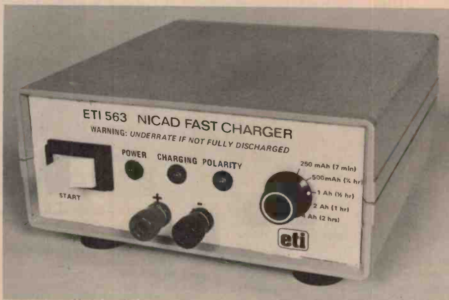
The completed project was housed in a smart PacTec case. Front panel is Scotchcal and will be available from the usual sources (see Shoparound on page 61).
