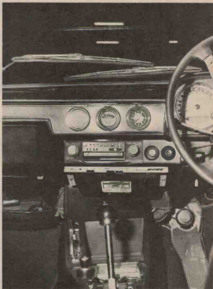
The Bose 1401 booster/equaliser is extraordinarily slim and mounts easily under a dashboard without being at all obtrusive.
