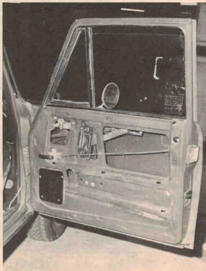
Chipboard is secured to the door panel and the speaker mounts on this. The door cavity may be stuffed with sound absorbent material to improve results.
