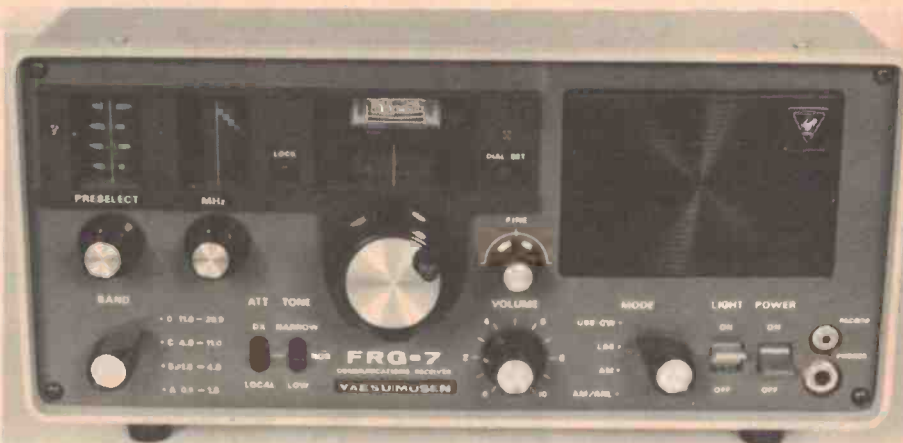
The Yaesu FRG-7 is a solid-state general coverage receiver employing the drift-cancelling "Wadley Loop" front end. It sells for around $350-$400 new, about $100 less second-hand.
