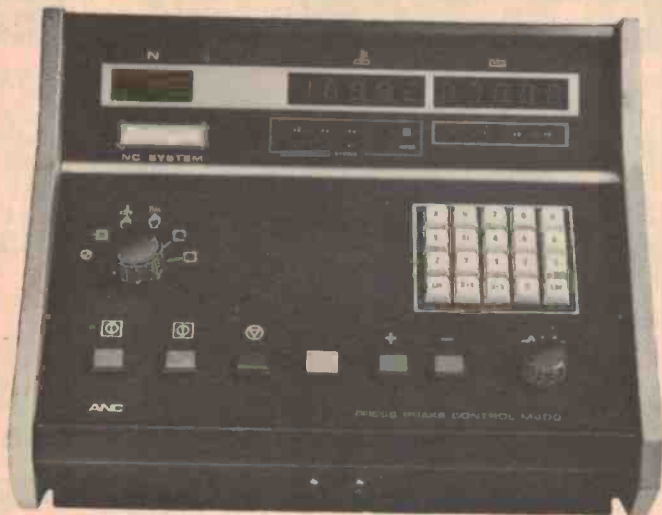
The ANC microprocessor press brake controller. The machine is programmed by the operator using a test piece, working from engineering drawings of the required plate shape.
