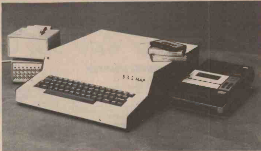
The Mini-Map shown with the input box and printer (sitting atop the input box). Any of the readily-available portable cassette players may be used with the system.
