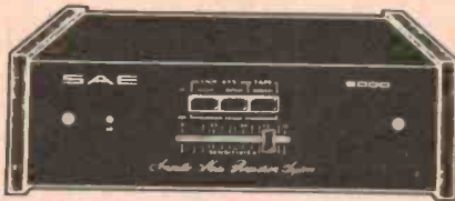
SAE 5000. Impulse noise reduction system: This is a specifically designed unit to reduce the "click" and "pop" (impulse noise) which are present in phonograph records and other programme sources.
