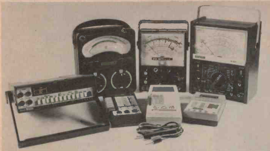
A multitude of multimeters! Analogue types lined up at the rear: from left to right, Avometer 8, Dick Smith's Q1140 and the Sanwa N-501. Front row digitals: from left to right, the Fluke 8600A portable bench DMM, Data Precision 935, Fluke 8020A and Tandy's Micronta 22-197. The latter three are low cost hand held models featuring liquid crystal displays.
