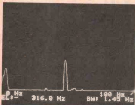
Second harmonic distortion performance as shown by the spectrum analyser.
