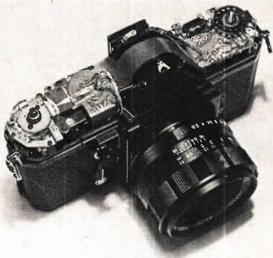
Fig. 9. The Yashica Electro AX is a fully automatic SLR with manual override. The camera has a flexible printed circuit wiring harness which can be seen at top.
