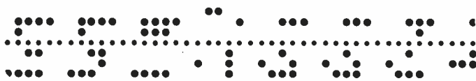
Fig. 2. Section of 8-hole punched tape. Two rows on the wider side of the central sprocket holes are not used in this data.
