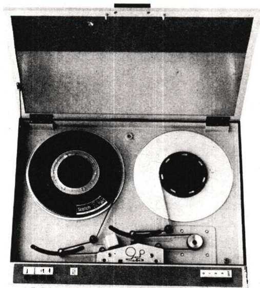
Fig. 15. The Hewlett-Packard 7970 magnetic tape unit designed as a peripheral to EDP systems.
