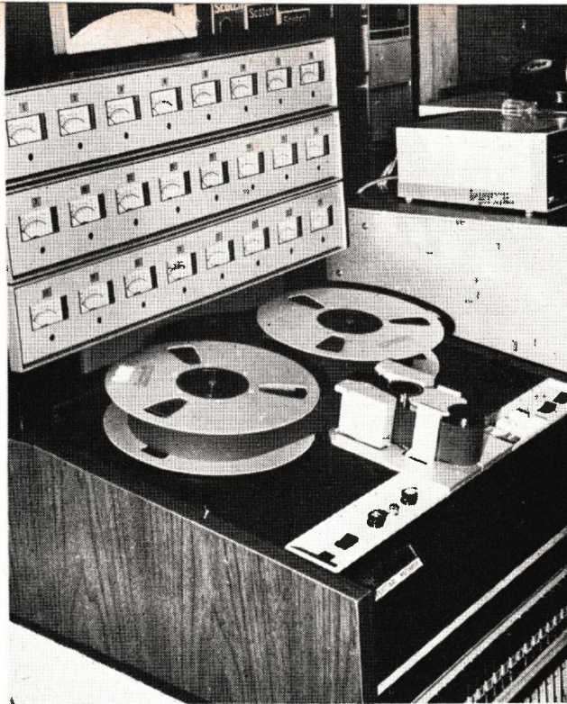
Fig. 4, 24 channel multitrack recorder utilising two-inch wide tape (manufactured by 3M)
