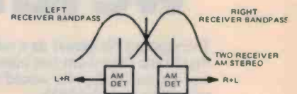
Fig. 4b. The stereo signal from the Kahn transmitter can also be picked up by two mono receivers, one tuned a little high, the other a little low.
