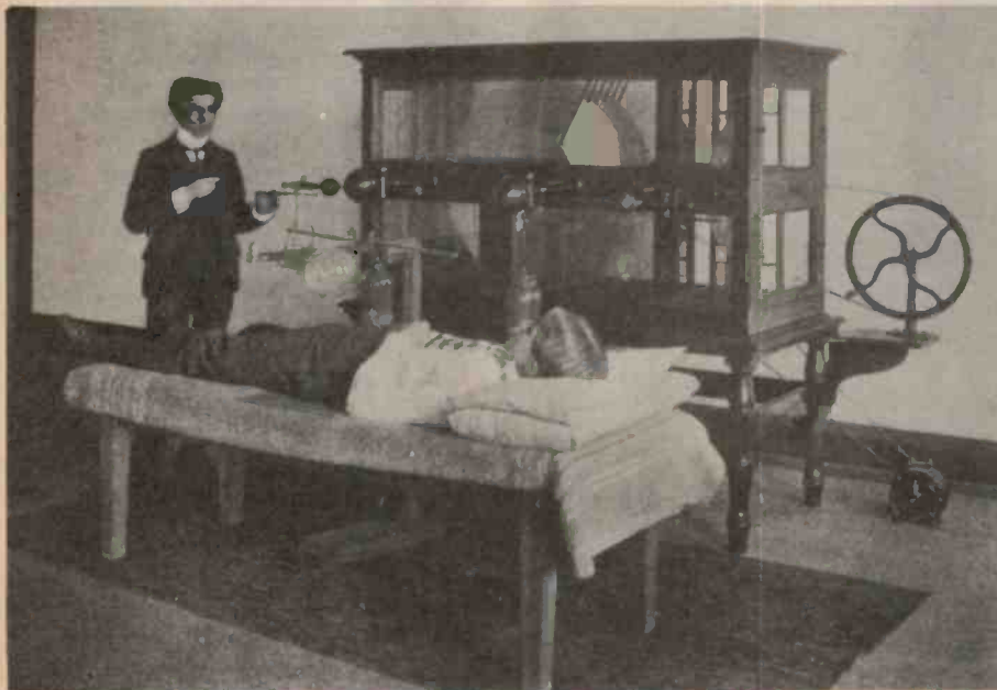
Fig. 7. Complete X-ray apparatus in use in America around 1900. Note the lack of safety devices and precautions.
