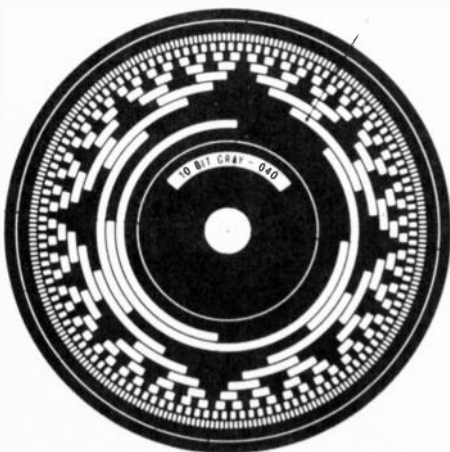
Fig. 5. The absolute digital code disc acts as a store of the angular value of displacement. It is interrogated as though it were a register whose value is read optically across a radial line.
