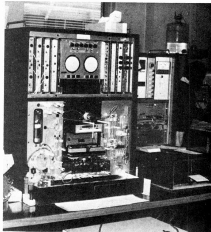
Fig. 8. Particles, blood cells in this case, pass through the small orifice (shown under the eyeglass) producing pulses that are counted. This is the basis of the Coulter Counter.
