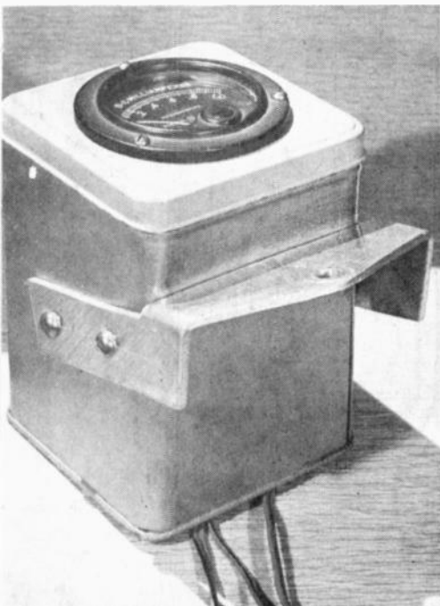
Fig. 1. The meter section may be attached to the handlebars by a bracket held by the handlebar pinch bolt. (meter dial is seen here before re-calibration).
