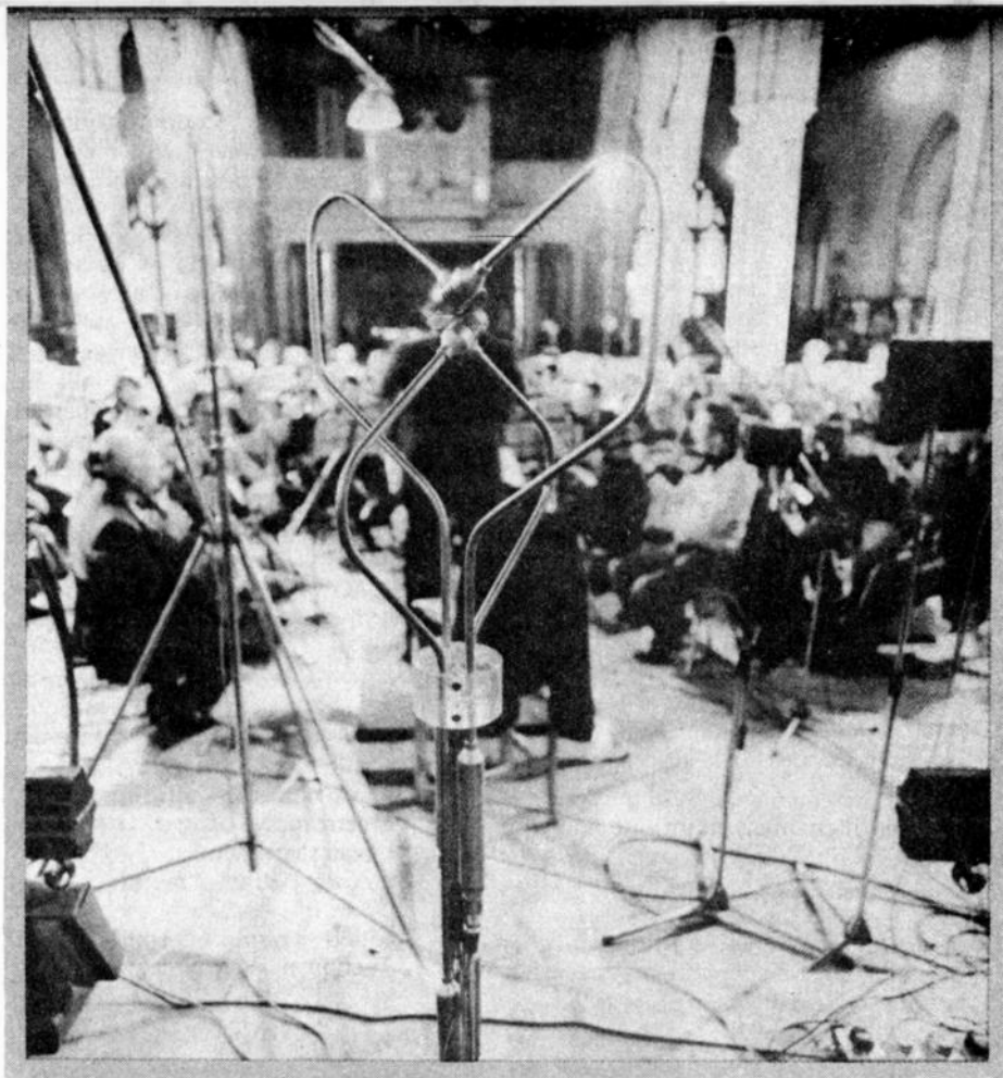
◀ Here the tetrahedral microphone array used for ambisonic recording is used to capture the direct and reverberant sound field in St. Giles' Church, in the city of London.
