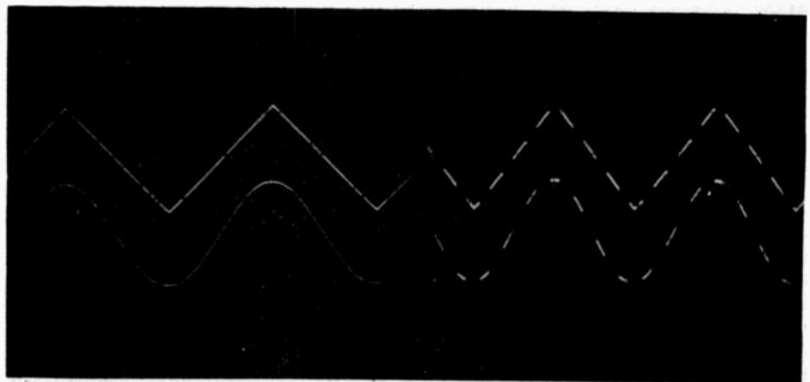
Fig.4a. Two signals, correctly displayed using the dual beam adaptor.
