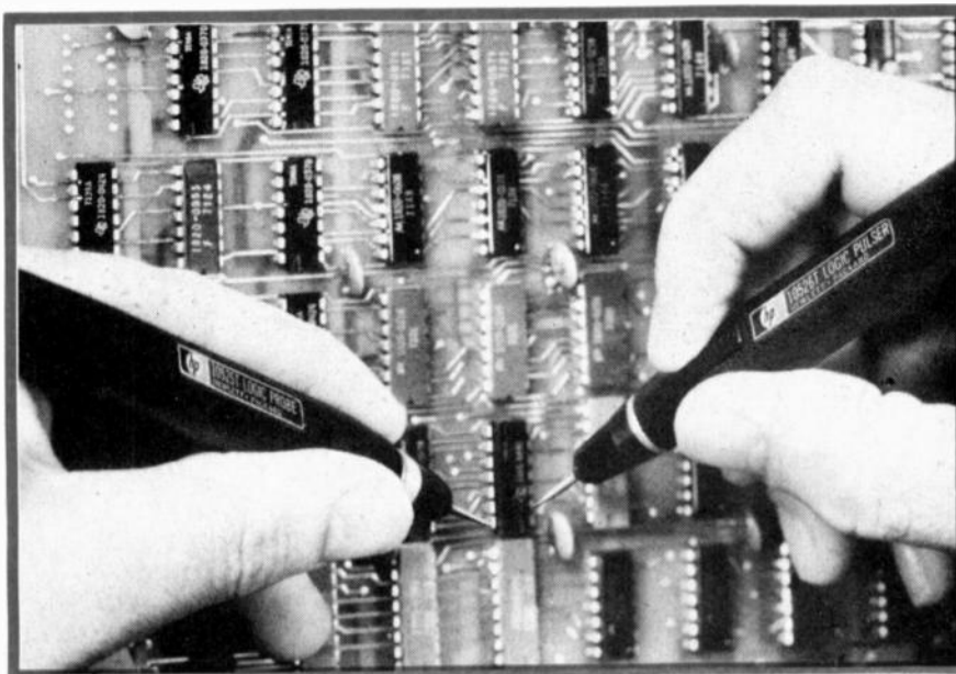
Here, a Hewlett-Packard logic probe is being used in conjunction with a logic pulser.
